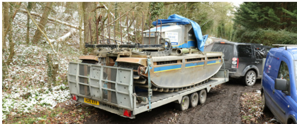
The two weeks before Easter saw a hired Truxor multi-purpose amphibious machine hired from Land & Water for silt and reed removal on the Loxwood section. Above: The machine being delivered at Roger Dimmick Lane.
