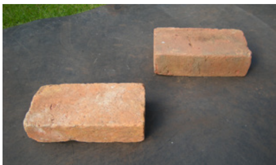
Examples of more than 200 original canal bricks from the downstream face of Gosden Aqueduct that the Midweek Working Party retrieved from the Cranleigh Waters river in late August. These hand-thrown bricks are quite heavy and surprisingly precise for their manufacture date of c.1815. They will help with repairs to the aqueduct.
