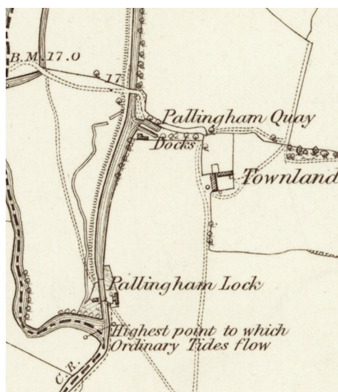
This early OS map shows the location of Pallingham Docks and Bridge. Mention is made in P.A.L Vine's Lost Route to the Sea that the docks were the only spot on the route between the Wey and the Arun where repairs to barges took place. Vine also notes that the barge Active , the last owned by Bramley wharfinger, lockkeeper and coal merchant William Stanton, was under repair at the docks in August 1870.
