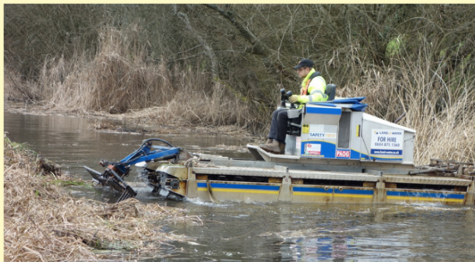
A hired-in Truxor has been put to good use at Drungewick to clear the proliferation of reeds. They have grown in the time the section has been closed to boats while volunteers worked on the leaks at Long Meadow and repaired Drungewick Lock. The machine was also used for some desilting around Baldwin's Knob Lock.
