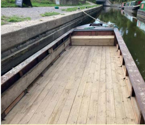
Above: The Canal Maintenance Unit did a great job of replacing the deck of May Upton. Right: BKL is just big enough for Wasp and May Upton at the same time.
