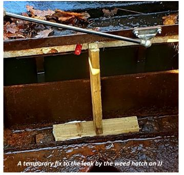
leak just in front of her weed hatch developed, which the new pump (1,100 galls or 4.9 tons per hour) just about coped with. John Reynolds stuck a piece of Blu Tack in the leaking 9mm hole which staunched the flow, and Ian, Brian and I came the next day to effect more permanent repairs. With underwater sealant on a piece of wood lodged over John's Blu Tack (still holding out the water) and jammed in by another piece of wood, the leak was deemed temporarily dealt with.
