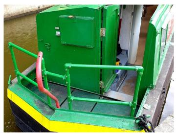
The big job on *Zachariah Keppel* was the construction and fitting of an after rail to stop the skipper falling overboard.
