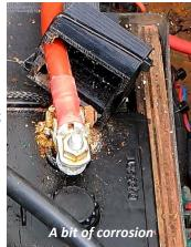
situation. A new clamp and the tightening of the top nut seems to have cured the problem, although eventually we will need a new, larger battery and heavier leads to the thruster unit.
