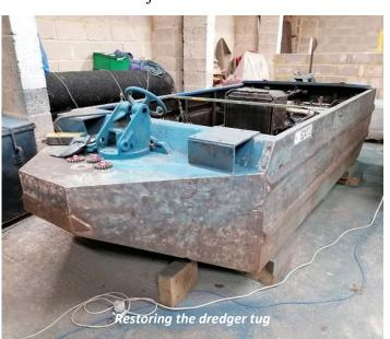
We also assisted the Dredging Team with their laborious task of wire brushing the hull of the dredger tug to strip it back to bare metal, in the first step of its renovation. Due to Health and Safety considerations, wire brushing with power tools is restricted to just 30 minutes per person per day, so it is a slow job but progress is being made. There is still much work to be done on the renovation and any offers of help would be gratefully received by the Dredging Team.
