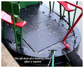
coats of our ample stock of black bitumastic paint. We still have to rub down, prime and paint the sides above the waterline and slip her to paint her bottom when we can get her down to the slipway.
