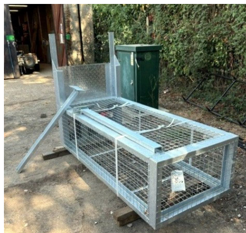
Pump cage galvanised and ready to go
