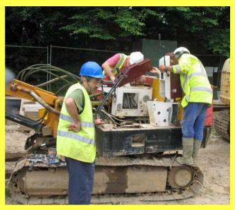
Hanix cab off - now find the leaking pipe
